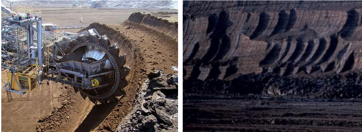
Figure 3. Mining process using bucket wheel excavators [3]
