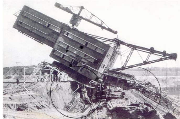
Figure 7. Tilt of chain excavator due to slope sliding [1]
