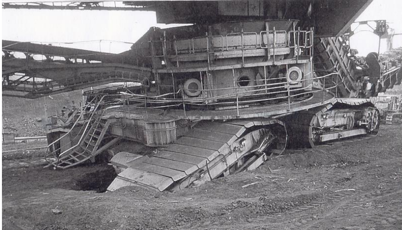
Figure 9. Caving of caterpillar vehicle [1]
