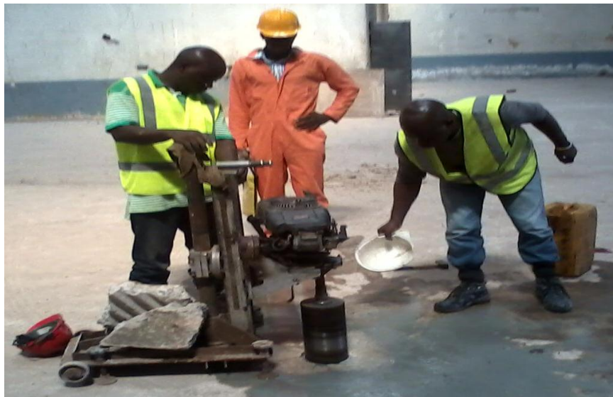
Figure 2.0: Plate Showing a Typical Core Drilling Machine (Source: INTECON PARTNERSHIP LTD –IPL.)
