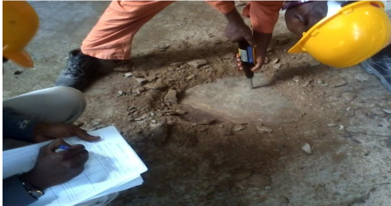
Figure 3.0: Plate showing a typical the use of the Rebound Hammer. (Source: IPL.)
