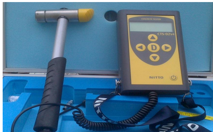
Figure 4.0: Concrete Tester and Surveyor CTS and Hammer Unit. (Source: IPL.)
